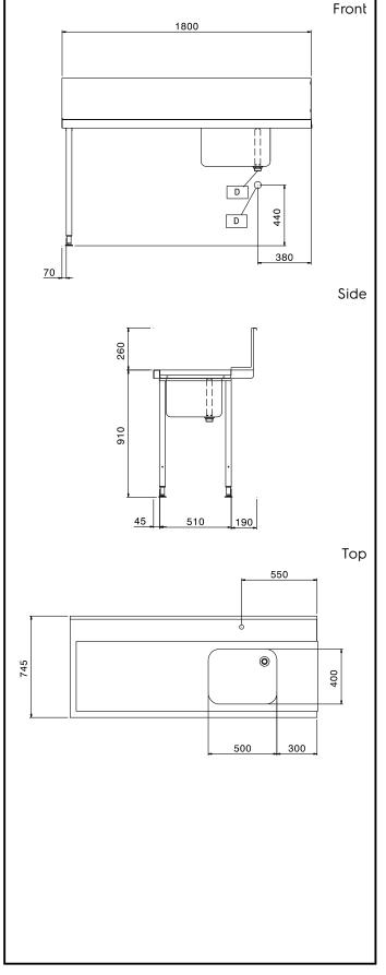
Handling System for Hood type Pre-wash Table with Bowl Left to Right, 1800mm
